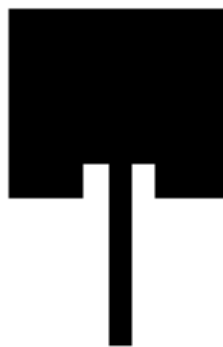
Fig. 2 - Geometry of Rectangular Antenna
